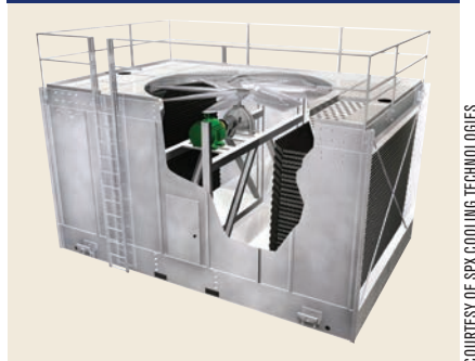
FIGURE 6 Crossflow; water flows down through the fill from the hot water basin on top, air flows horizontally across the water path.
