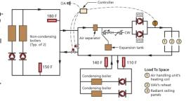
Based on OAT, the system's supply water temperature shall be adjusted. When it is relatively warm outside, the supply water temperature can be reduced and the system can maintain space design conditions with lower supply water temperature, during which the condensing boilers will operate in condensing mode and water will circulate through the secondary loop only.
